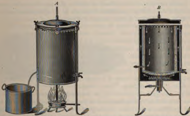
Fig. 39.—Lautenschläger's steam sterilizer for dressings: A, Exterior view; B, cross-section.
